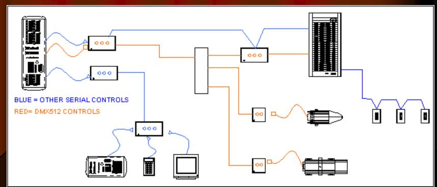
Adding RDM to today's DMX512 system will reduce the set-up time needed to configure the system and reduce the number of proprietary serial interfaces.
